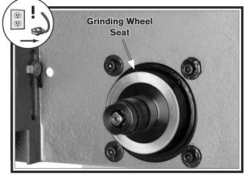
Figure 26. Wheel mounting hub.
